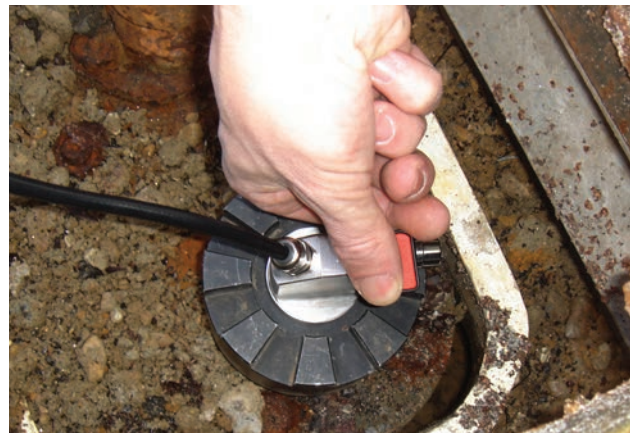
Leak on 800mm diameter iron main over 276 metres (London, UK)
